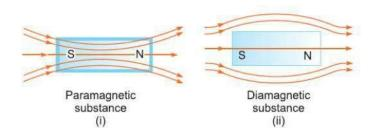
19. The material which has relative permeabilities slightly greater one are paramagnetic whereas the material which has relative permeabilities slightly lesser than one are diamagnetic.
